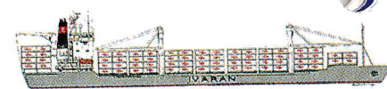
SAN FERNANDO - Containervessel, delivery August 1996. About 20,000 dwt/1,512 TEUs (cellular). Speed: about 20 knots.
