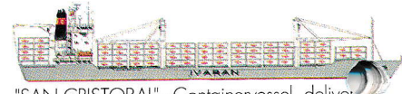
"SAN CRISTOBAL" - Containervessel, delivery December 1995. About 20,000 dwt/1,512 TEUs (cellular). Speed: about 20 knots.
