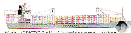
"SAN CRISTOBAL" - Containervessel, delivery December 1995. About 20,000 dwt/1,512 TEUs (cellular). Speed: about 20 knots.
