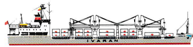
"SANTA FE" - Semi-containervessel, built 1978. 14.770 dwt/447 TEUs + 2 coiled/coated deep tanks for liquid cargo, of 11.410 cbft each. Speed: about 16,5 knots. Accommodation for 12 passengers.
