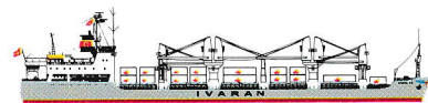
"SALVADOR" — Semi-containervessel, built 1978. 14.770 dwt/447 TEUs + 2 coiled/coated deep tanks for liquid cargo, of 11.410 cbft each. Speed: about 16,5 knots. Accommodation for 12 passengers.
