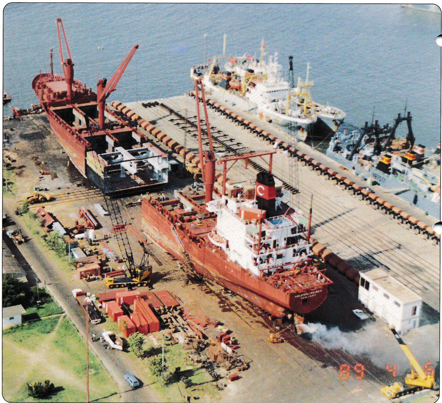
M/S San Diego being jumboized in Buenos Aires.
